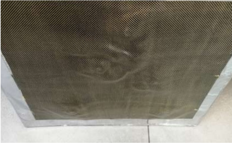
Aramid test plate at different velocity. No penetration at 444 m/s
