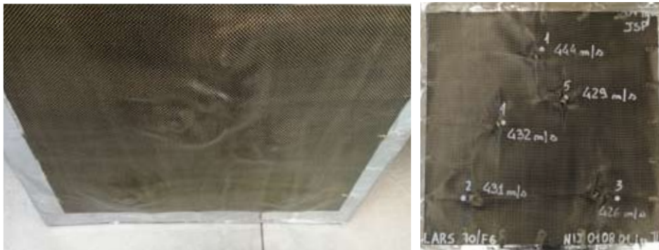
Aramid test plate at different velocity. No penetration at 444 m/s
